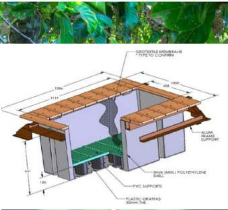
▶ Diagram of prototype floating mangrove barge (by Mourjan Marinas)
